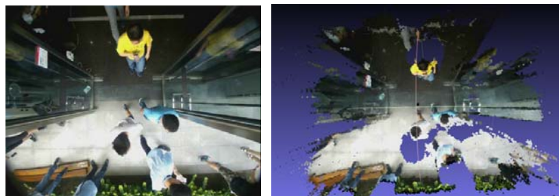
Figure 4 The Image From The Left Lens And The Corresponded Top View of 3D Image
